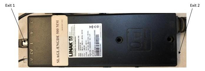
It is very important to use the correct exit points on the control box. If 2 actuators are connected then use exit points 1 and 2. If 3 actuators are connected, then use exit points 1, 2 and 3. If you use exit points 1 and 4, the control box will not function.
